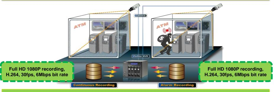
Uses one/same video stream for both alarm and regular recording at same resolution and FPS at ALL times.
