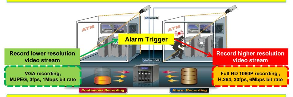
Dynamically switch to record higher resolution and FPS on alarm trigger. Small bit rate stream for Regular Recording; high bit rate stream for Alarm Recording. ---> Higher demand for HDD storage space ONLY when an event occurs!
