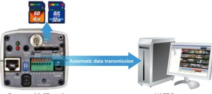
Camera with SD card for backup recording VAST Server
