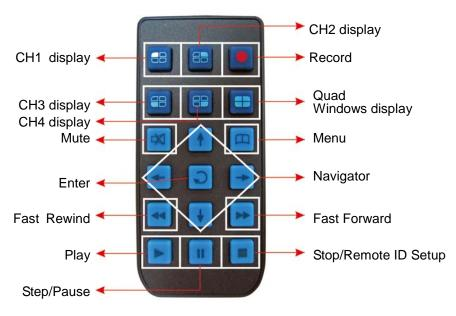
**★**Under the LIVE screen, press fast forward button twice within 1 second, can switch GUI interface.
