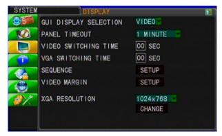
GUI Display GUI display mode can be VIDEO or VGA.
