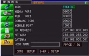
■ Mode Set the connection method. Set: Static IP, DHCP, PPPoE.
