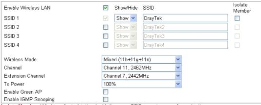
Isolate Member: Wireless clients (stations) with the same SSID cannot access for each other.
