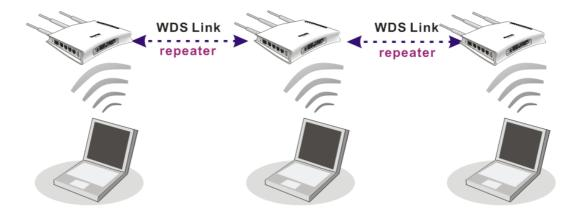
In **Bridge** mode, the router will connect to up to four Vigor2130 which use the same mode, and all wired Ethernet clients of every Vigor2130 will be connected together. You can use this mode to connect a network to other networks which is physically isolated. Please note that when you set to this mode, Vigor2130 will not accept regular wireless clients anymore.
