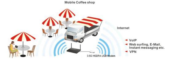
After connecting into the router, 3G USB Modem will be regarded as the second WAN port. However, the original Ethernet WAN still can be used and Load-Balance can be done in the router. Besides, 3G USB Modem also can be used as backup device. Therefore, when WAN is not available, the router will use 3.5G for supporting automatically. The supported 3G USB
