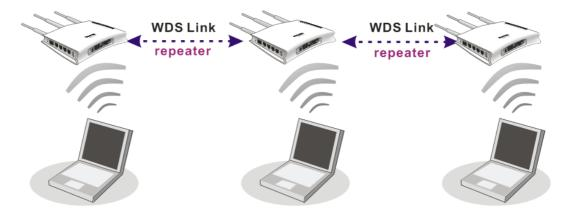
In **Bridge** mode, the router will connect to up to four Vigor2130 which use the same mode, and all wired Ethernet clients of every Vigor2130 will be connected together. You can use this mode to connect a network to other networks which is physically isolated. Please note that when you set to this mode, Vigor2130 will not accept regular wireless clients anymore.
