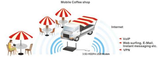
After connecting into the router, 3G USB Modem will be regarded as the second WAN port. However, the original Ethernet WAN still can be used and Load-Balance can be done in the router. Besides, 3G USB Modem also can be used as backup device. Therefore, when WAN is not available, the router will use 3.5G for supporting automatically. The supported 3G USB Modem will be listed on DrayTek web site. Please visit www.draytek.com for more detailed information.
