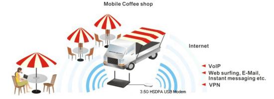
After connecting into the router, 3G USB Modem will be regarded as the backup WAN port. Therefore, when WAN is not available, the router will use 3.5G for supporting automatically. The supported 3G USB Modem will be listed on DrayTek web site. Please visit www.draytek.com for more detailed information.
