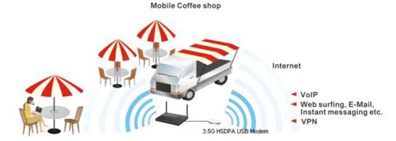
After connecting into the router, 3G USB Modem will be regarded as the backup WAN port. Therefore, when WAN is not available, the router will use 3.5G for supporting automatically. The supported 3G USB Modem will be listed on DrayTek web site. Please visit www.draytek.com for more detailed information.
