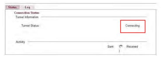
When the router detects all the information, the screen will be shown as follows. One set of **TSPC prefix** and **prefix length** will be obtained after the connection between TSPC and Tunnel broker built.
