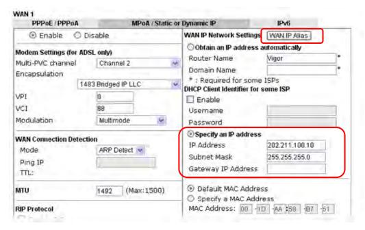
Click the **WAN IP Alias** button to configure the other P address which is 202.211.100.11. Make sure **Join IP NAT Pool** is not checked. Click **OK** to save the settings.
