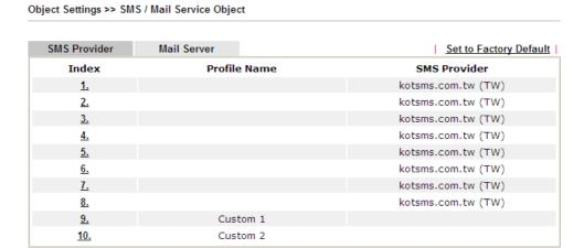
Index 1 to Index 8 allows you to choose the built-in SMS service provider. If the SMS service provider is not on the list, you can configure Index 9 and Index 10 to add the new service provider to Vigor router.
