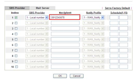
9. Click **OK** to save the settings. Later, if one of the WAN connections fails in your router, the system will send out SMS to the phone number specified. If the router has only one WAN interface, the system will send out SMS to the phone number while reconnecting the WAN interface successfully.
