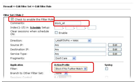
**Note:** In default, the router will check the packets starting with Set 2, Filter Rule 2 to Filter Rule 7. If **Block If No Further Match** for is selected for **Filter**, the firewall of the router would check the packets with the rules starting from Rule 3 to Rule 7. The packets not matching with the rules will be processed according to Rule 2.
