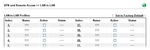
3. Click any index number to open the configuration page. Type a name which is easy for identification for such profile (in this case, type *VPN Client*), and check the box of **Enable This Profile**. For such Vigor router will be set as a **client**, the call direction shall be set as **Dial-out**. Check the box of **Always on** for a permanent VPN connection.
