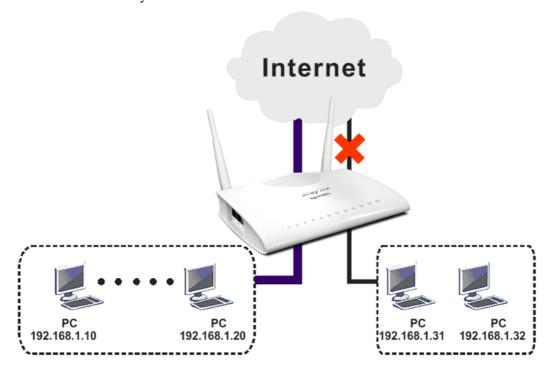
The way we can use is to set two rules under **Firewall**. For **Rule 1** of **Set 2** under **Firewall>>Filter Setup** is used as the default setting, we has to create a new rule starting from Filter Rule 2 of Set 2.
