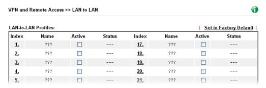
3. Click any index number to open the configuration page. Type a name which is easy for identification for such profile (in this case, type *VPN Server*), and check the box of **Enable This Profile**. For Vigor router will be set as a **server**, the call direction shall be set as **Dial-in** and set 0 as **Idle Timeout**.
