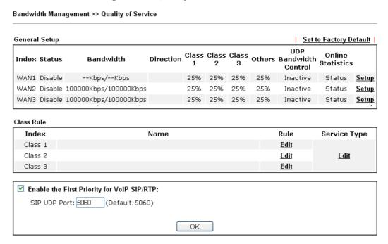
2. Click **Setup** link of WAN(1/2/3). Make sure the QoS Control on the left corner is checked. And select **BOTH** in **Direction**.
