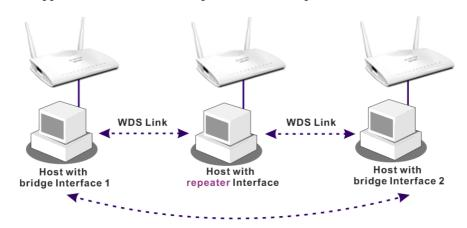
The major difference between these two modes is that: while in **Repeater** mode, the packets received from one peer AP can be repeated to another peer AP through WDS links. Yet in **Bridge** mode, packets received from a WDS link will only be forwarded to local wired or wireless hosts. In other words, only Repeater mode can do WDS-to-WDS packet forwarding.
