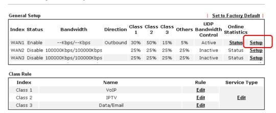
In the Setup page, check the box of Enable the QoS Control. Type 30, 50 and 15 in the boxes for VoIP, IPTV and Data/Email respectively. Check the box of Enable UDP Bandwidth Control.
