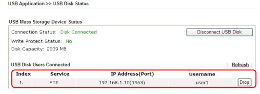
Now, users in LAN of Vigor2710 can access into the USB storage device by typing ftp://192.168.1.1 on any browser. They can add or remove files / directories, depending on the Access Rule for FTP account settings in USB Application >> USB User Management.
