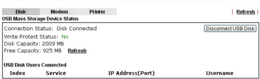
Note: If the write protect switch of USB disk is turned on, the USB disk is in READ-ONLY mode. No data can be written to it.
