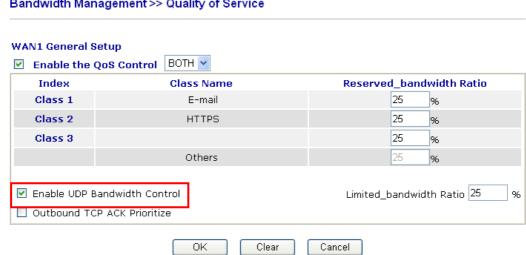
8. If the worker has connected to the headquarter using host to host VPN tunnel. (Please refer to Chapter 3 VPN for detail instruction), he may set up an index for it. Enter the Class Name of Index 3. In this index, he will set reserved bandwidth for 1 VPN tunnel.
