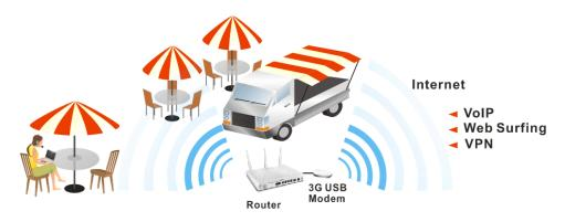
After connecting into the router, 3G USB Modem will be regarded as the third WAN port. However, the original WAN1 and WAN2 still can be used and Load-Balance can be done in the router. Besides, 3G USB Modem in WAN3 also can be used as backup device. Therefore, when WAN1 and WAN2 are not available, the router will use 3.5G for supporting automatically. The supported 3G USB Modem will be listed on DrayTek web site. Please visit www.draytek.com for more detailed information.
