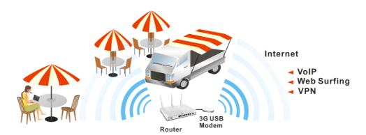
After connecting into the router, 3G/4G USB Modem will be regarded as the third WAN port. However, the original WAN1 and WAN2 still can be used and Load-Balance can be done in the router. Besides, 3G/4G USB Modem in WAN3 also can be used as backup device. Therefore, when WAN1 and WAN2 are not available, the router will use 3.5G for supporting automatically. The supported 3G/4G USB Modem will be listed on DrayTek web site. Please visit www.draytek.com for more detailed information.
