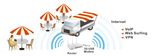
After connecting into the router, 3G USB Modem will be regarded as the third WAN port. However, the original WAN1 and WAN2 still can be used and Load-Balance can be done in the router. Besides, 3G USB Modem in WAN3 also can be used as backup device. Therefore, when WAN1 and WAN2 are not available, the router will use 3.5G for supporting automatically. The supported 3G USB Modem will be listed on DrayTek web site. Please visit www.draytek.com for more detailed information.
