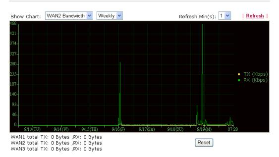
The horizontal axis represents time. Yet the vertical axis has different meanings. For WAN1/WAN2/WAN3 Bandwidth chart, the numbers displayed on vertical axis represent the numbers of the transmitted and received packets in the past.
