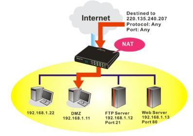
The security properties of NAT are somewhat bypassed if you set up DMZ host. We suggest you to add additional filter rules or a secondary firewall.
