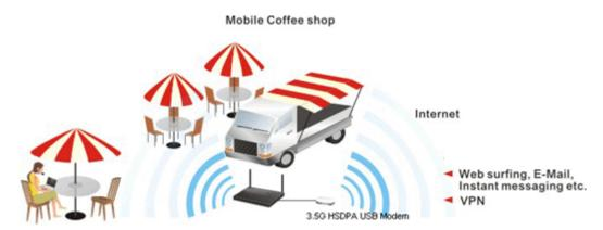
After connecting into the router, 3G USB Modem will be regarded as the third WAN port. However, the original Ethernet WAN1/WAN2 still can be used and Load-Balance can be done in the router. Besides, 3G USB Modem in WAN3 also can be used as backup device.
