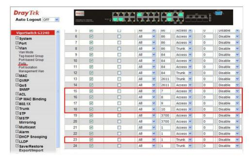
4. After finishing the above configuration, the equipment connecting to VigorSwitch Port 15, 16, 17 and 18 can get the corresponding IP address(es) of the network segment.
