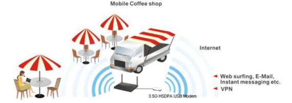
After connecting into the router, 3G/4G USB Modem will be regarded as the third WAN port. However, the original Ethernet WAN1/WAN2 still can be used and Load-Balance can be done in the router. Besides, 3G/4G USB Modem in WAN3 also can be used as backup device. Therefore, when WAN1/WAN2 is not available, the router will use 3.5G for supporting automatically. The supported 3G USB Modem will be listed on Draytek web site. Please visit www.draytek.com for more detailed information.
