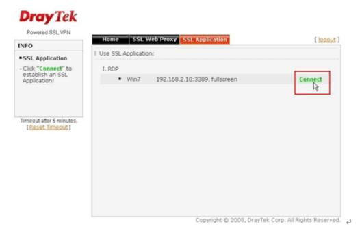
9. After that, you can access into Windows 7 via a browser. Note the message below the window. In which, TLS means Transport Layer Security.
