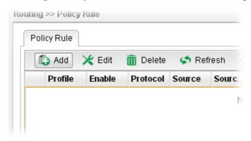
3. In the following page, type a name for such profile; check **Enable**; choose **Subnet** as **Destination Type**; type 203.65.1.35 as IP address; choose **Load Balance Pool** as **Out-going Rule**; choose WAN1 as the **Load Balance Rule**; click **Disable** for **Failover to Next Rule**.
