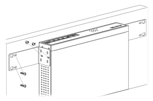
Then, continue to fasten the screws on the other side of the router and the wall with other screws.
