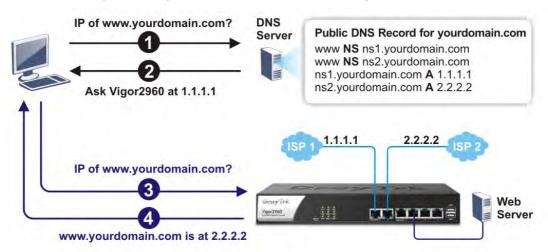
Open WAN>>Load Balance and click the Inbound Load Balance tab.
