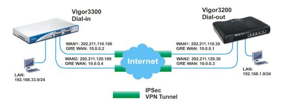
At present, Vigor3200 just supports one VPN trunk group with two members for the same VPN network pair. In this case, the VPN trunk is built for 192.168.1.0/24 <-> 192.168.33.0/24. In other word, although Vigor3200 supports 4 WAN connections, it just allows you to use 2 VPN connections over two WAN ports for one VPN trunk group between the networks 192.168.1.0/24 and 192.168.33.0/24.
