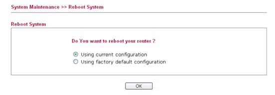
If you want to reboot the modem using the current configuration, check **Using current configuration** and click **OK**. To reset the modem settings to default values, check **Using factory default configuration** and click **OK**. The modem will take 5 seconds to reboot the system.
