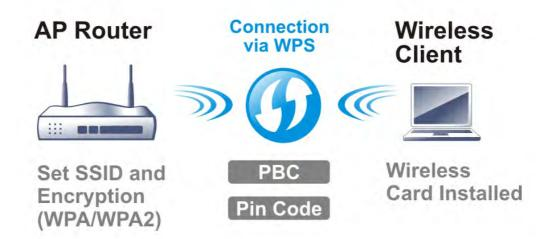
It is the simplest way to build connection between wireless network clients and VigorAP 900. Users do not need to select any encryption mode and type any long encryption passphrase to setup a wireless client every time. He/she only needs to press a button on wireless client, and WPS will connect for client and VigorAP 900 automatically.
