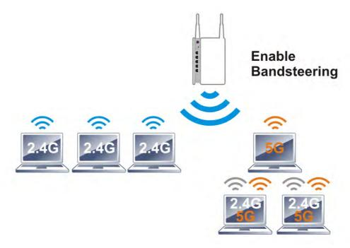
**Note**: To make Band Steering work successfully, SSID and security on 2.4GHz also MUST be broadcasted on 5GHz.
