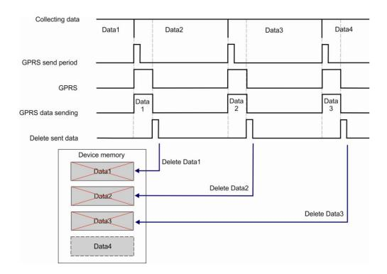
Periodical data saving: after given time to send data, device connects to server through GPRS and sends data. Right after that device deletes sent data.
