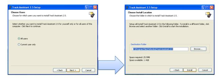
6. Please connect device and press *OK* if setup wizard will ask to connect device to computer. If you press *Cancel* device drivers will not be installed. Press *Continue anyway* if hardware installation window pops out.
