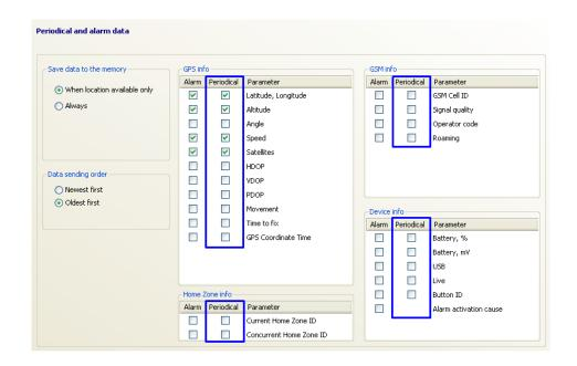
**Alarm data** is sent in case alarm was activated. Data can be chosen: *Device configuration*  $\rightarrow$  *Connections and Data*  $\rightarrow$  *Periodical and alarm data*. In order to send alarm data it has to be configured using Track Assistant software: *Device configuration*  $\rightarrow$  *Connection and Data*  $\rightarrow$  *GPRS and Server columns*.
