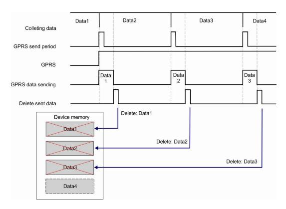
Periodical data sending when Hold server connection alive parameter is enabled
