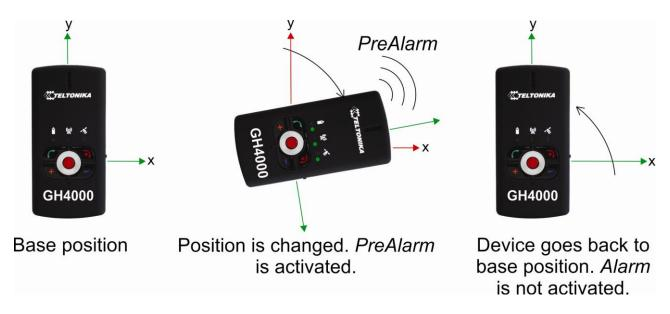
When *Man – down* function is enabled and device position is changed more than 45 degrees *PreAlarm* is activated. Device does not go back to its true (base) position until *PreAlarm* time runs out – alarm is activated.
