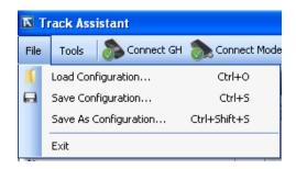
File option lets you load configuration file \_\_\_\_.afg, save configuration as a file, save configuration as a different file.
