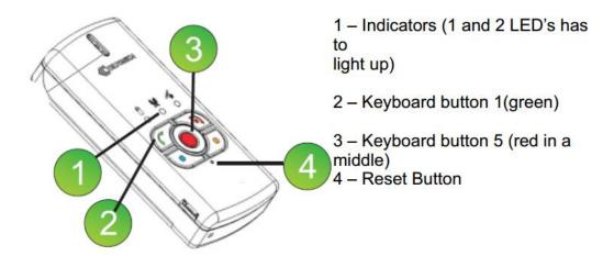
b) While holding pressed green and red buttons, connect GH4000 to computer via USB cable. Make sure GH4000 is in Firmware update mode (battery's (1) and GSM's (2) LEDs should light up green). Do not connect GH4000 to Track Assistant!
