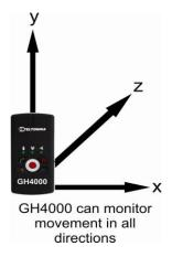
There are a lot of side effects (e. g. vibration) which can affect measurements of accelerometer. That's why GH4000 has an integrated filter, which helps to reduce the influence of such factors. Device reaction when Man – Down is enabled is displayed in pictures below:
