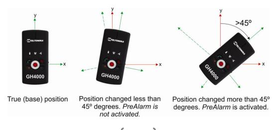
*Man – down* function is enabled and device position is changed more than 45 degrees *PreAlarm* is activated. If device goes back to its true (base) position until *PreAlarm* time runs out – alarm is not activated. Device continues monitoring its position.
