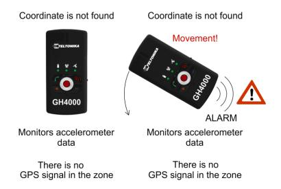
Parking function is activated. There is no movement. GH4000 does not find new coordinate. Device goes to movement (accelerometer) monitoring mode. PreAlarm is activated when movement is recorded. Alarm is activated after PreAlarm time runs out. Couple scenarios, when device is not able to get new coordinate, are displayed below.
