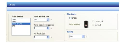
This is main Alarm configuration section. Configurable parameters are explained in a table below:
