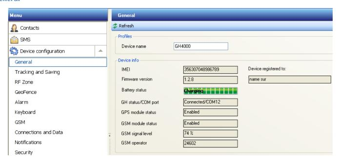
General info tab shows such device information: IMEI, firmware version, battery status, GH status/COM port, GPS module status, GSM module status, GSM signal level, GSM operator code.
