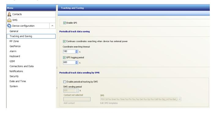
In this submenu GPS data logging settings can be controlled. In order to save changed configuration to device *Apply* button has to be pressed.
