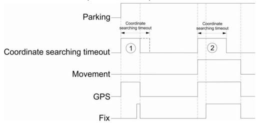
Operation of parking function when new coordinates are found and device does not leave the zone.
