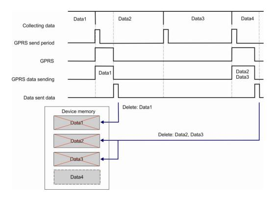
Periodical data sending when device fails to send data (Data2)
