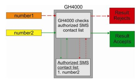
Operation of GH4000 when call security is enabled
